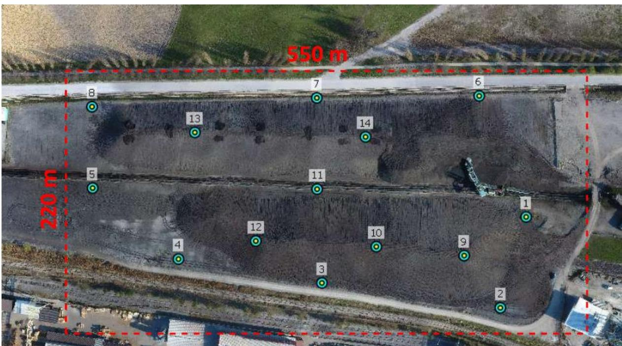
In case of uneven (or rugged) terrain it is highly recommended to place GCPs on both lowest and highest points of your area of interest.
