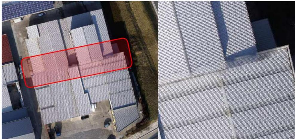
To eliminate the over-the-building image stitching we advise you to have the whole building on a single image. First, perform your mission at 80 m AGL, then manually trigger a few nadir images from a higher AGL (120 m above the object, for example) to get the whole object in one image. That enables you to recalculate the area with - or/and around - the building.
