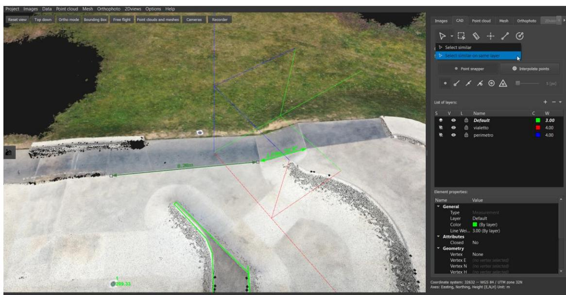
All data of selected object or layer are displayed in **Element properties** window of **working panel**. There you can change its **colour**, **line type** or **layer** by clicking on desired attribute and change it from available possibilities.
