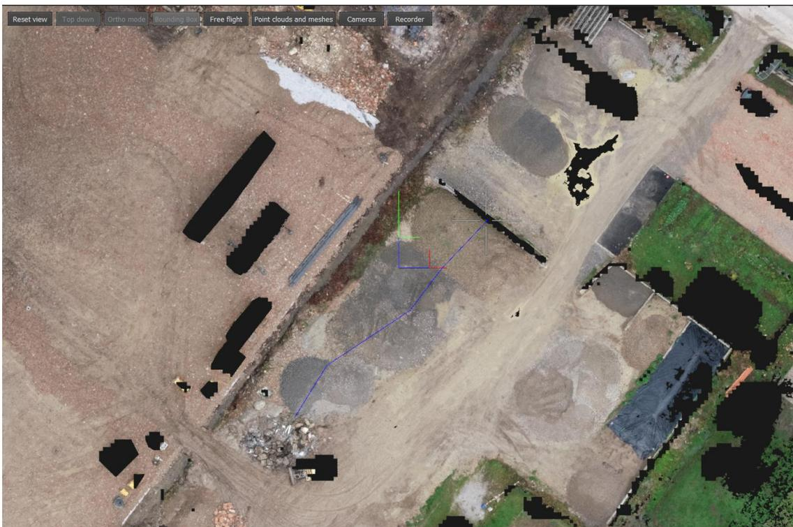
Calculated profile is displayed on the Point cloud in both 2D and 3D or on the mesh (purple line).
