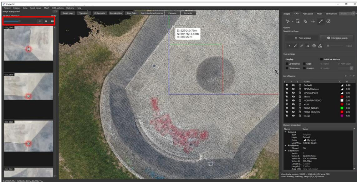
Use the photos to position the cursor on the desired point, using the different angles to ensure that the selected position is the correct one.
