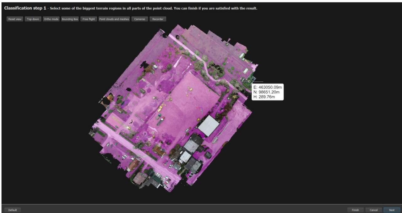
Click on Continue to allow the software to refine the search for points to be classified. At this point you will move on to the second classification step with which to further refine the classification, if you notice any parts of the terrain that are poorly classified.
