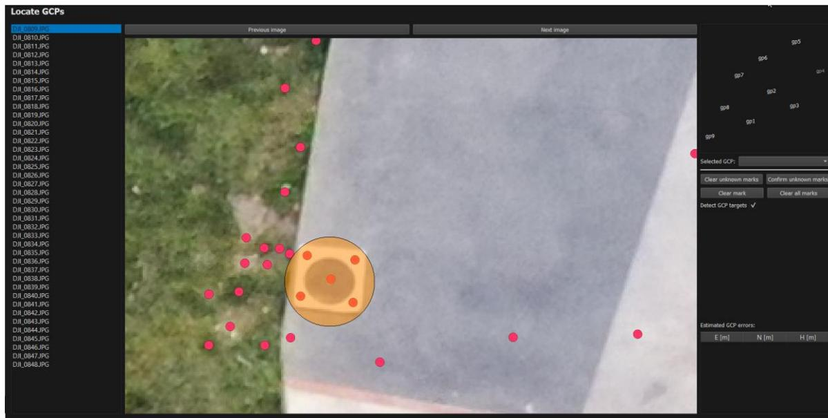
Continue by **selecting additional two** GCPs from other segments of your project area. When you select the third ground control point the automatic recognition for all other GCPs will start. Three marked GCPs remain orange coloured while automatically found GCPs are now coloured green and the names of all GCPs are identified.
